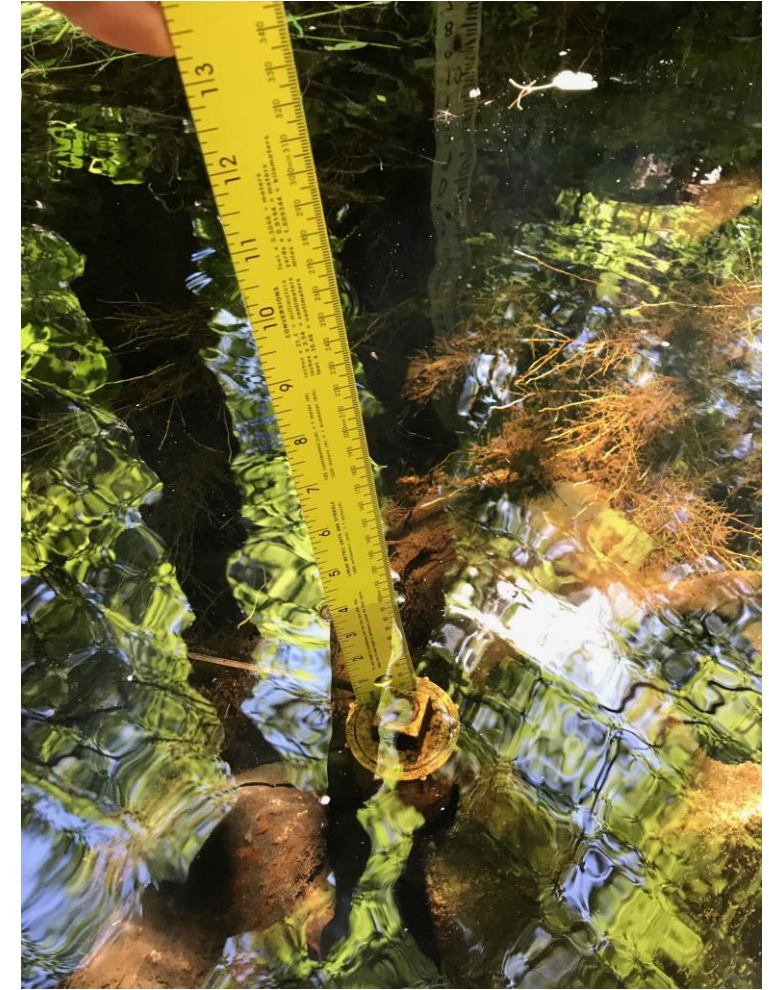
Measuring water height (stage) above pressure logger at downstream of Drowns Dam.
